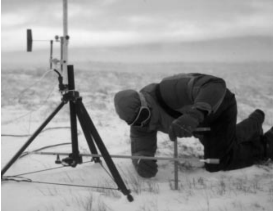
Figure 2. Photograph of the senior author checking the height of the electric field mill at the end of experiments on 7 January 1994. Wind sensors (background) were on a short mast downwind and to one side of the electric field measurement.
