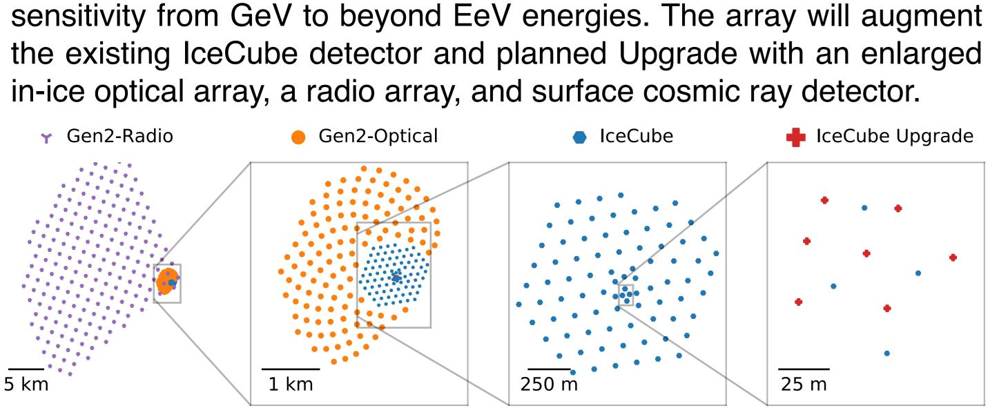
1 km<sup>3</sup>, 86 strings, most with 125 m lateral spacing 60 DOMs/string with 17 m spacing, completed 2011
