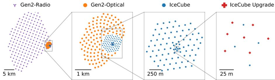
**IceCube:** 1 km<sup>3</sup>, 86 strings, most with 125 m lateral spacing
