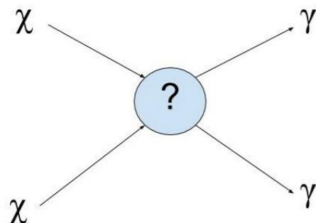
Peak in the  $\gamma$  energy distribution at the WIMP mass (“ $\gamma$ -ray line”) would be clear signal for DM annihilations.
