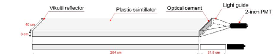
Figure 2: Schematic view of muon detector materials and assembly part
