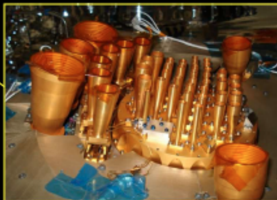
LFI Radiometers 30-70 GHz, T = 20\text{ K}
