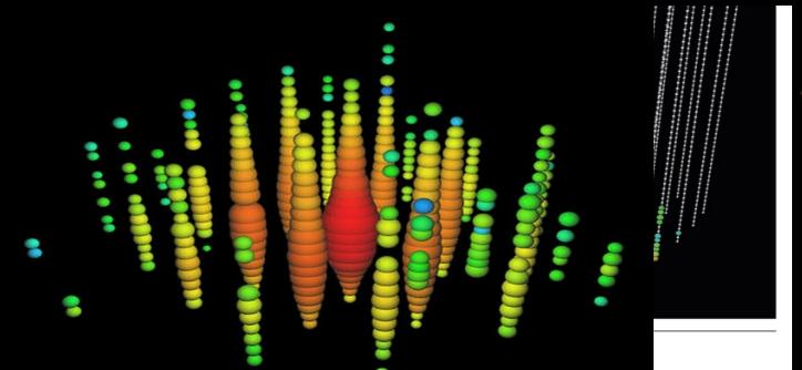
A 250 TeV neutrino interaction in the interaction point (bottom), a large interaction with a muon produced in the interaction point (top). The direction of the muon indicates the original neutrino.
