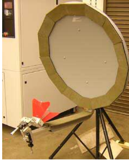
Figure 4.12: Parabolic reflector dish with Eccosorb on edges.
