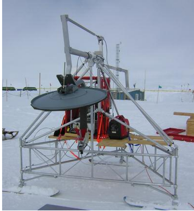
Figure 4.13: Antenna and antenna pointing system.
