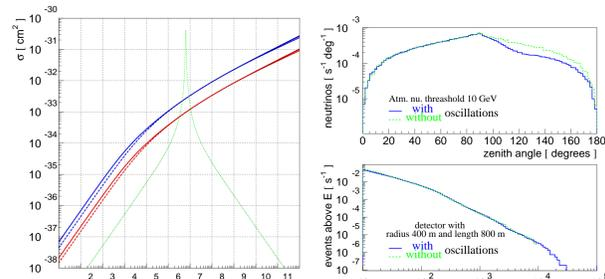
Simulated neutrino cross sections: higher blue curves are CC, lower red curves are NC; solid are  $\nu$ , dashed are  $\bar{\nu}$ ; green dotted is  $\bar{\nu}_e e^- \rightarrow W^-$ . Neutrino flavor oscillations: muon events. Since latitude-dependent geomagnetic cut-off is not calculated, a fixed 10 GeV cutoff is applied.
