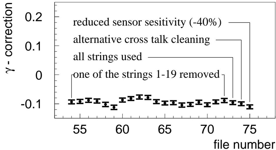
results demonstrated remarkable stability with respect to detector configuration changes and choice of the ice model
