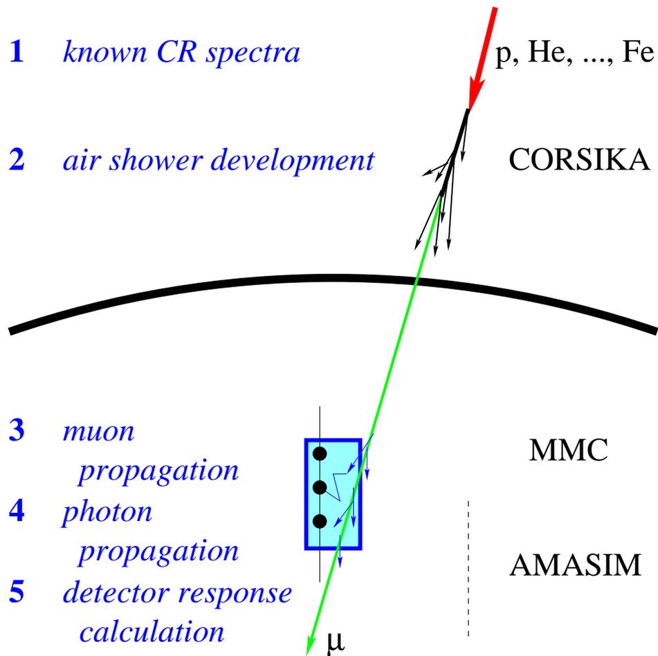
To simulate background an air shower generator (CORSIKA) is run, then muons are propagated (with MMC), and then the photons are propagated and detector response is evaluated (with AMASIM).
