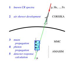
To simulate background one needs to run an air shower generator (CORSIKA), muon propagator (MMC) and then propagate photons and evaluate detector response (AMASIM).
