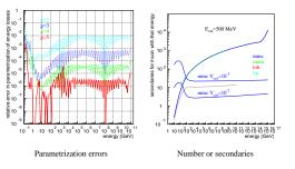
MMC employs a very customizable parametrization scheme. It uses both polynomial and rational function interpolations spanned over varying number of points (5 by default). The algorithm is very stable and allows calculations to be performed in an energy range even bigger than physically interesting without losing precision (over 15 orders of magnitude in energy). Other muon propagation codes have limited energy resolution and smaller precision in only part of MMC's region of applicability.
