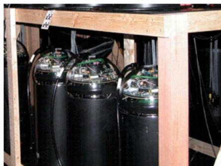
(b) Three DOMs set up for testing. The wooden supports of the upper shelf can be seen at the edges of the photo.
