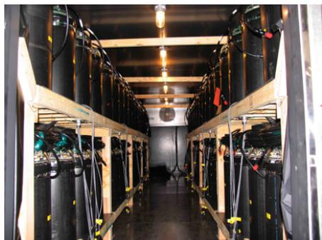
(a) The entire inside of the DOM testing freezer in Madison. Two wooden shelves on each side of the central aisle each contain 15 DOMs on stands, for a total of 60 DOMs.
