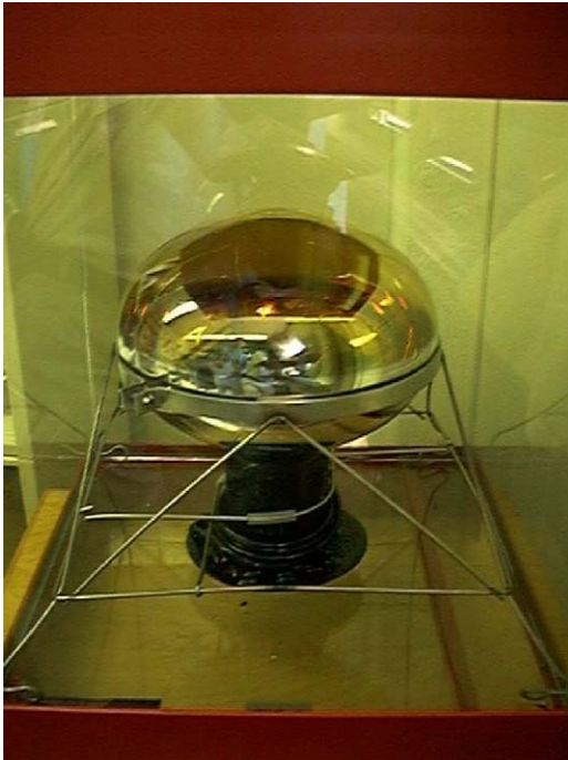
Fig. 1. A typical phototube used in the MiniBooNE detector: an 8 in. R1408 mounted on its wire frame. The base is coated with Masterbond (as described in Section 2.1) before the PMT is installed into the detector.
