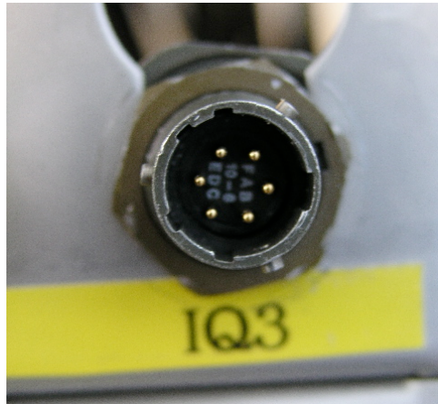
Figure 4: Wrong Connector on IQ3, JDR Cable, TCH End
