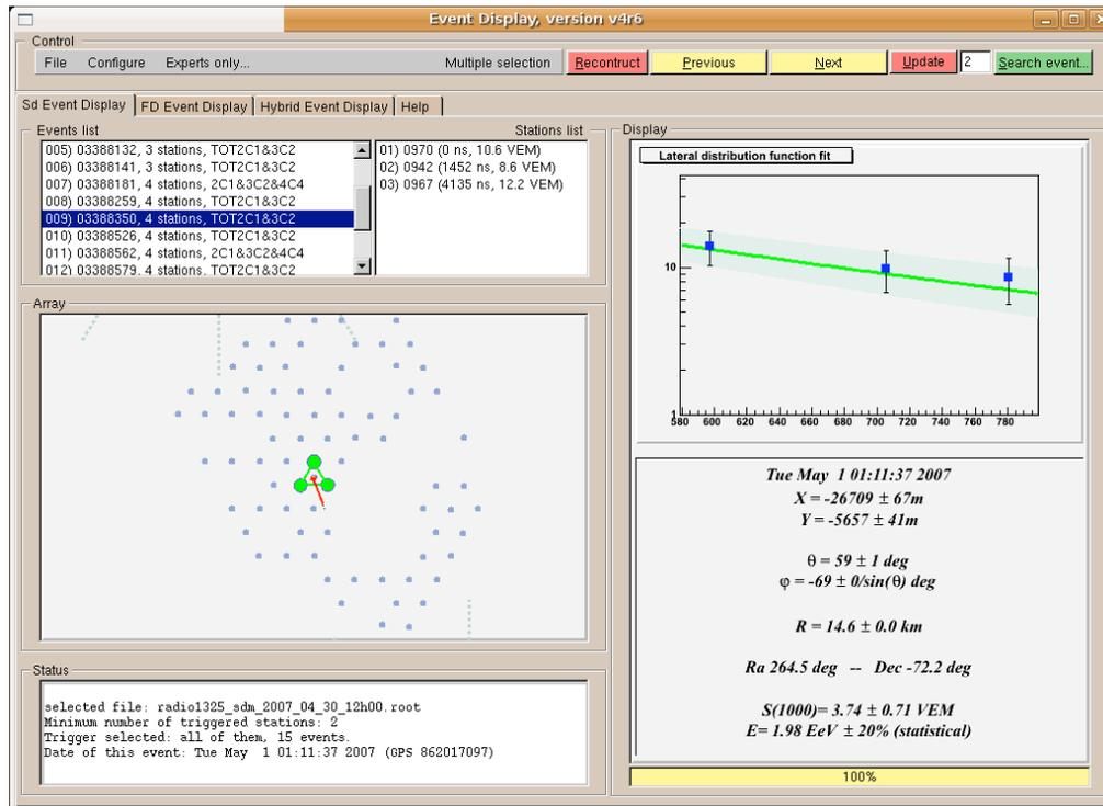
Auger SD display ( $E \sim 2 \text{ EeV}$ )
