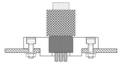
\*\*The purpose of this item is to keep the XSJJ Seacon connector thread from entering more than 1" depth below the top surface. The opening at the bottom may have the same diameter as the drill hole for tapping.
