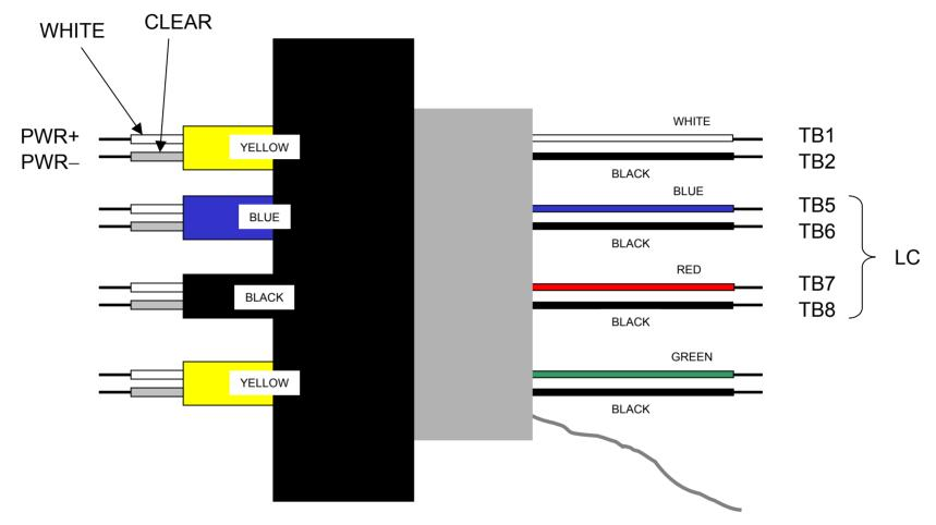
The drain wire is N/C including the mounting threads.
