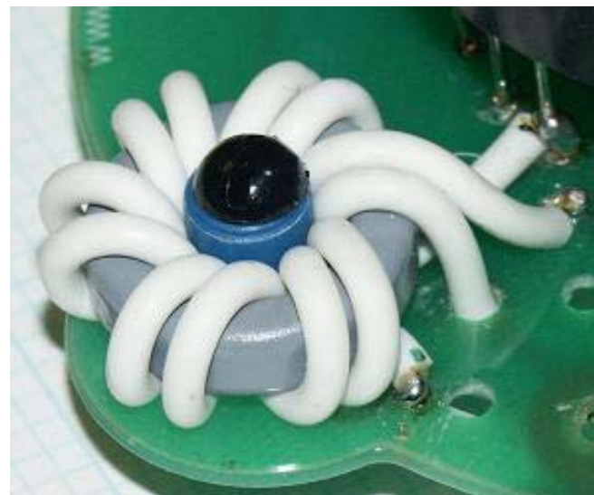
New Transformer 22 AWG silicone-insulated bifilar → Rated at 10kV
