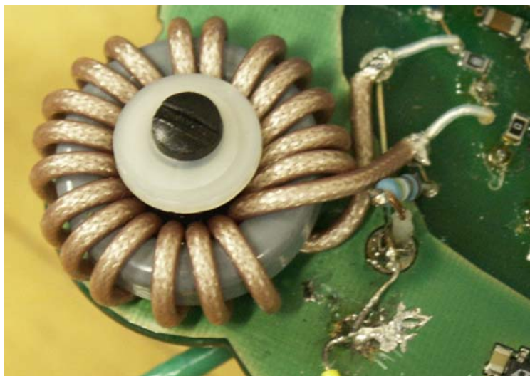
Old Transformer RG178 coaxial cable → Rated at 1000Vrms
