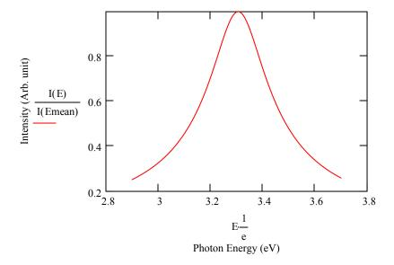
Optical output for IF=10 mA is Po = ~700uW at 25 degC (Rank 2 devices)
