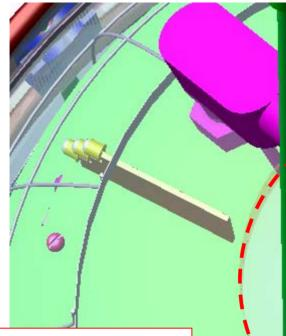
HV Generator Mounted on the bottom side of the daughter board. The coax comes straight up thru a hole in the daughter board.
