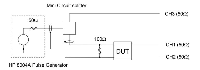
CH3  $\rightarrow$  Input pulse Trace "A" = (CH1 – CH2)  $\rightarrow$  Output pulse The output pulse was measured in a differential mode
