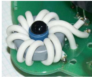
Figure 2 Sample transformer mounted on the PCB.
