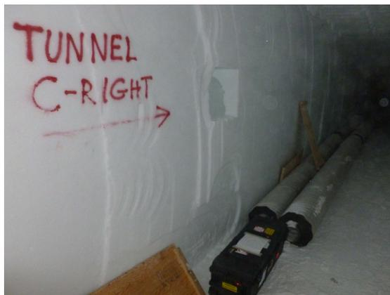
(d) Muon detector operating in tunnels at start of tunnel 'C' underneath Amundsen bust
